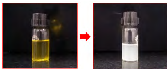
Figure 12. Synthesis of nanoparticles from CGM via antisolvent precipitation method: before and after
